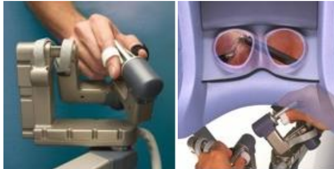
Figure 7 The da Vinci handle used to remotely move the instrument's tip ( http://www.intuitivesurgical.com )
